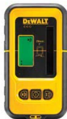
**WATERPROOF DIGITAL ROTARY LASER DETECTOR**
