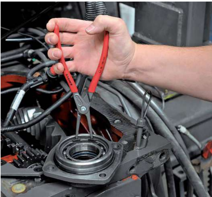
Sturdy, inserted tips: made from high-density spring steel
