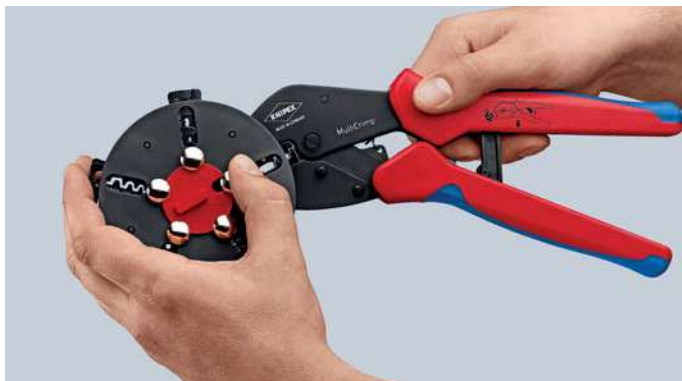
Changing the crimping dies: unlock the magazine position, take out the set of dies which the pliers have been pushed on
