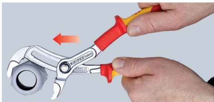
Quick setting without using a push-button
