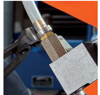
Sealing the hose connection on central lubrication
