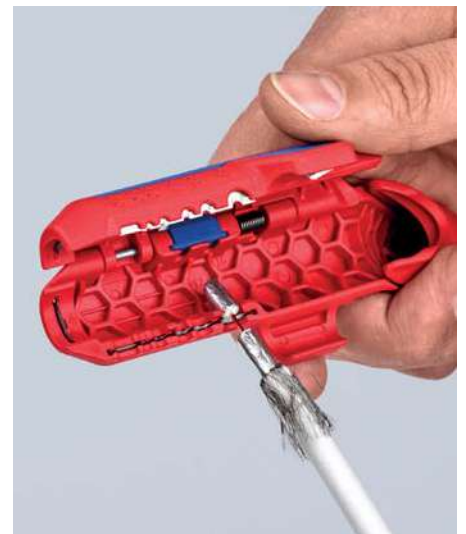
Stripping of a coax cable
