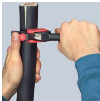
Turning the tool for circumferential cut
