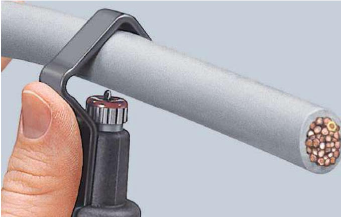
Setting the tool for circular cutting
